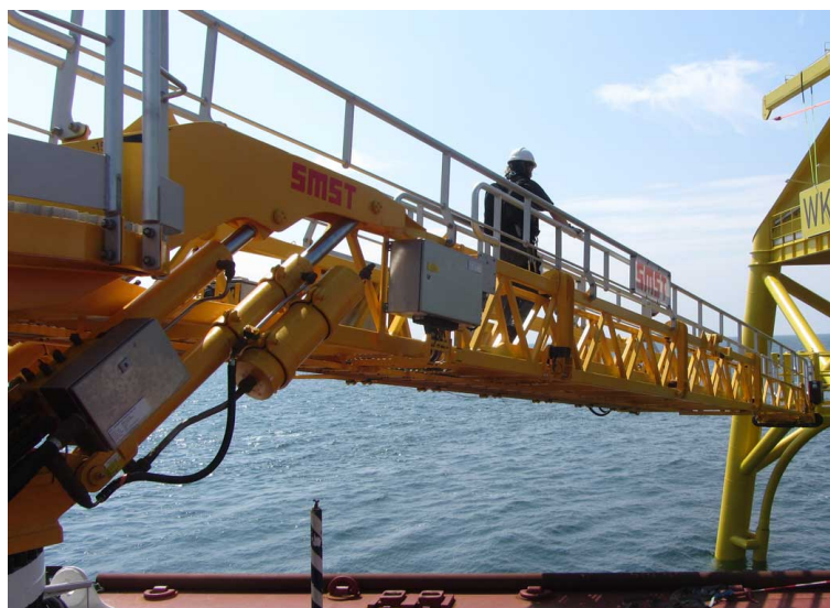
Figure 1: Motion compensated gangway (picture courtesy of SMST).
