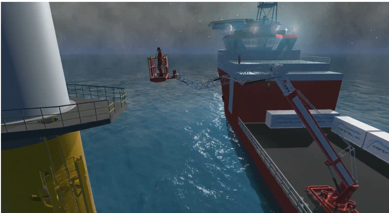
Figure 2: 3D real-time simulation of a motion compensated crane.
