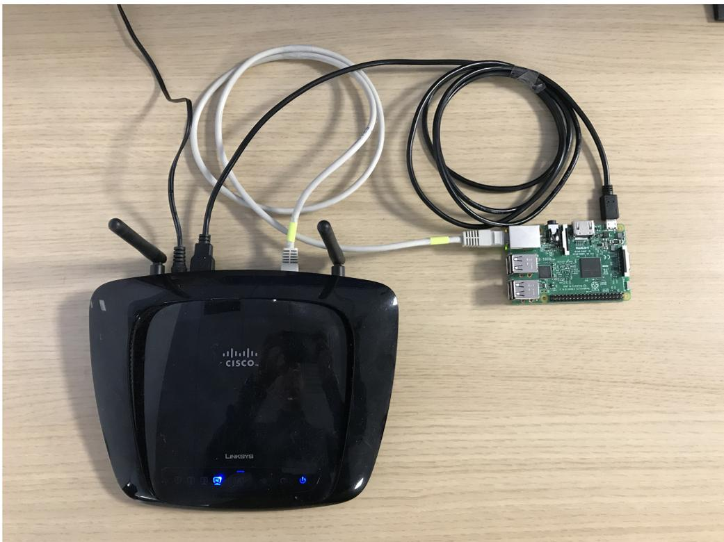
Figure 3: The Raspberry Pi 3 board used for HiL co-simulation.
