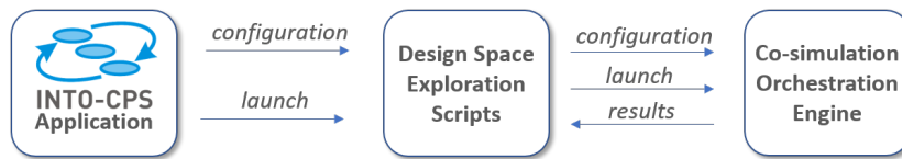
Figure 1: Outline connections between DSE and the INTO-CPS application and COE
